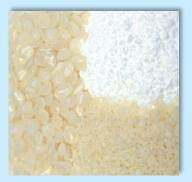
Zinc Stearate CM - this clear melt zinc stearate is one of the most widely used additives in the plastics field. It also serves as a lubricant or emulsifier in the toiletries and cosmetics areas, and can be used for mold release.
